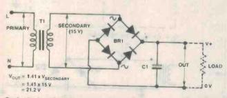
Basic single-ended supply using a bridge rectifier module.
