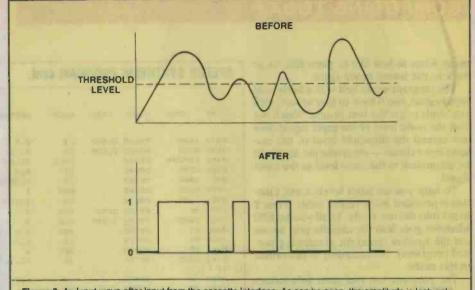
Figure 3. An Input wave after input from the cassette interface. As can be seen, the amplitude is lost, only the frequency remains. The output is 1 if the value of the wave is above the threshold level, 0 if not.
