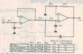
Fig 3b. Third order low-pass filter. To alter break frequency (in this case 1 kHz) scale resistors accordingly.
