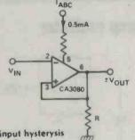
Transconductance type; input hysterysis levels = ±V<sub>OUT</sub>; V<sub>OUT</sub> = R x I<sub>ABC</sub>
