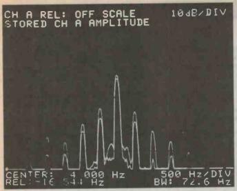
Shure Ultra 500 tested with TRR103 Test Record with 1000 and 1500 Hz twin tone at 31.5 and 40 cm/s maximum velocities.
