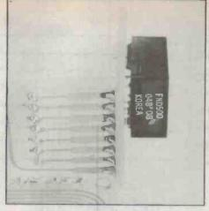
which is placed against the main board so that the edge connectors line up. They are fillet soldered at right angles.
