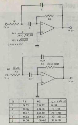
Fig 5. A multiple feedback bandpass filter. The centre circuit is normalised for 1 kHz. The table is the design table for this circuit. To change the design frequency change R1 and R2 by an equal factor.
