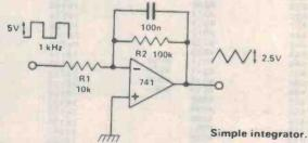
but not enormously. A good point about this integrator design is that it has a very low output impedance. You can put a load on the output and the opamp will still generate the same waveform—that's what is so nice about negative feedback.
