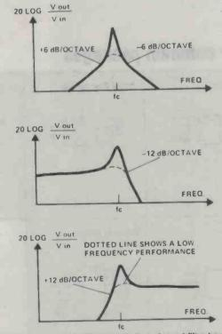
Fig 6b. The state variable filter is called a universal filter because it can give band-, low- and high-pass outputs — as shown above. Note that all these responses are second order.
