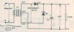
Basic single-ended supply using a centre-tapped transformer.
