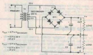
Basic dual supply using a bridge rectifier module.
