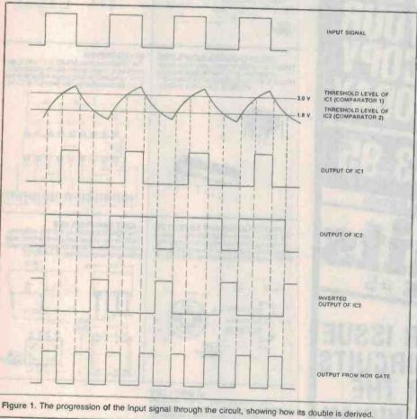
This project allows you to easily double clock frquencies or have a TTL signal and its double without dividing down.
