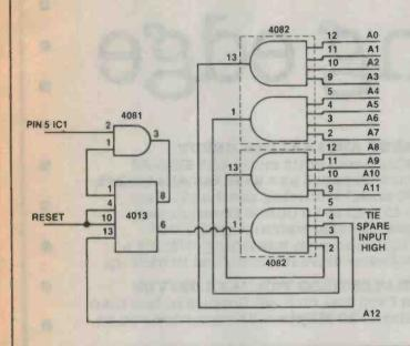
This circuit is a modification for the ETI-668 Microbee EPROM Burner by Tom Moffat and Geoff Nicholls. It saves manually switching between two 'halves' of a 2764.
